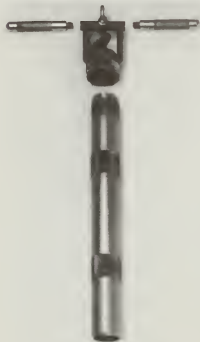
Figure 10-26 Hand-held sediment corer (courtesy Wildlife Supply Company)
